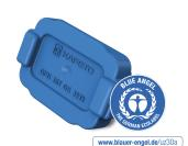
The GPN 367 C contact protection is used to protect TE connector housings (german) in low-voltage applications. Thanks to its internal clamping contour, the contact protection seals according to protection class IPX2. Its flat design allows it to be used in confined installation spaces. Additionally, the contact protection can be installed from either side.
